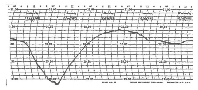
1. In the space below, make a table of the barometric pressures from the barograph at four hour intervals. Start the table at 8:00 am on Saturday and end with 8:00 am on Sunday. Record the barometric pressures to the nearest tenth of an inch.
