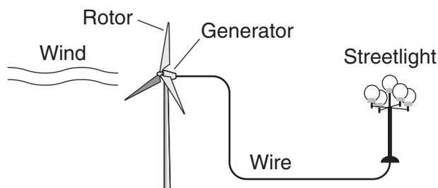
Which part of the system directly changes mechanical energy to electrical energy?
